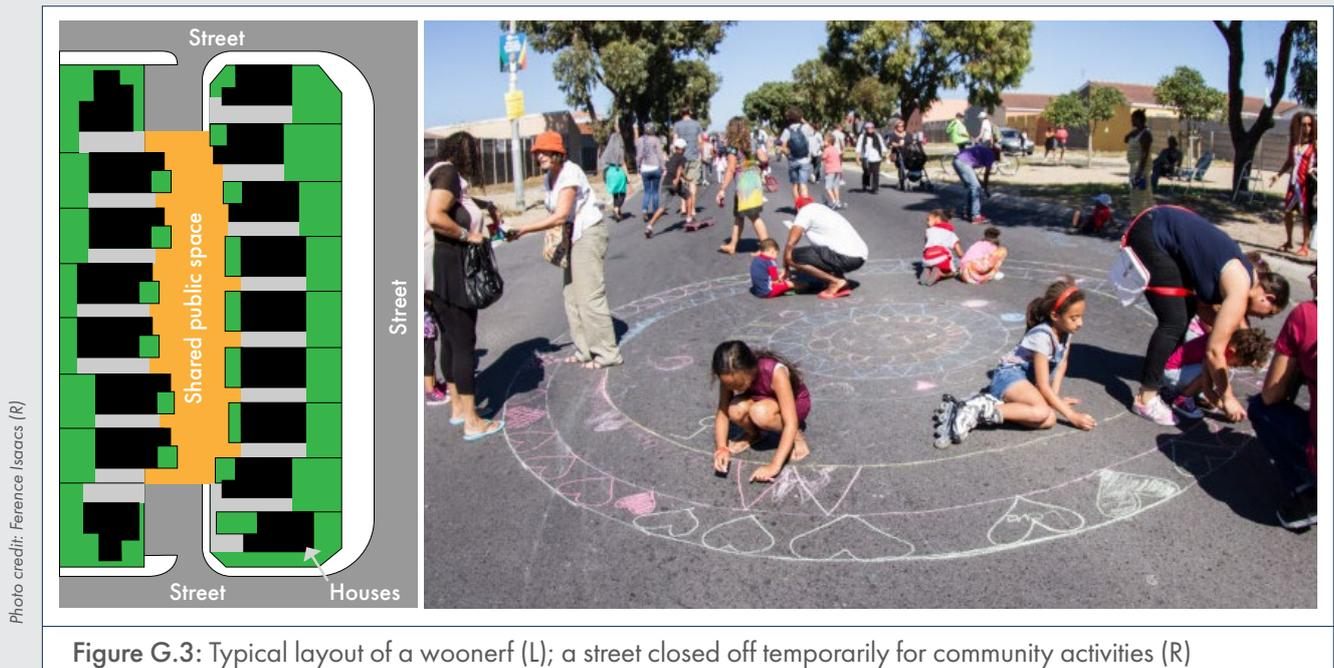
**Figure G.3:** Typical layout of a woonerf (L); a street closed off temporarily for community activities (R)
