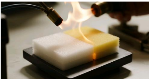
Aerogel materials feature low thermal conductivity, are non-combustible, and moisture-proof.
